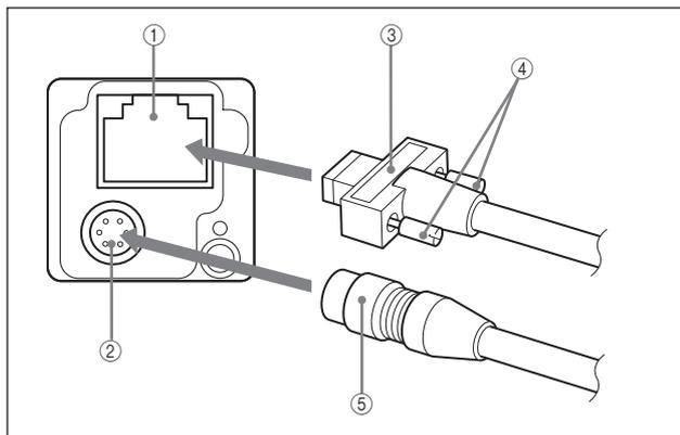
Connect the camera cable to the DC IN connector and connect the LAN cable to the RJ45 connector respectively. If you use a camera module interface board or a hub that supports PoE, you can operate the camera even if you do not connect the camera cable to the DC IN connector. When you connect the LAN cable with fastening screws, turn the two screws on the connector to secure the cable tightly.
