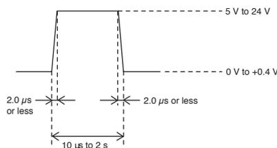
Trigger input polarity = Negative
